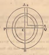
the pole : force of gravity at the equator :: 289 : 288. Suppose A B Q q a spheroid revolving, the lesser diameter P Q, and A C Q q c a a canal filled with water. Then the weight of the arm Q q c C : ditto of A a c C :: 288 : 289. The centrifugal force at the equator, therefore 1 suppose  $\frac{1}{2BQ}$  of the weight.
